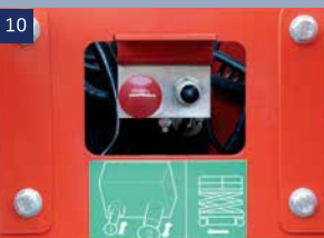
Manual release valve: When the machine doesn't work, you can push the machine after pressing this valve.
